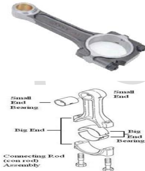
Fig: 1.3 Connecting Rod assembly with press fitted brass bush, Cap, Nuts and Bolts
